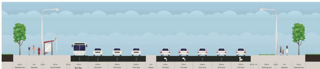
Figure 6-3: Arterial A2 – Recommended Cross-Section, Intersection
