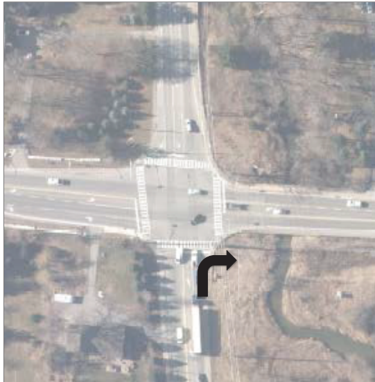
Alternative Solution #2 Additional Northbound Right Turn Lane
