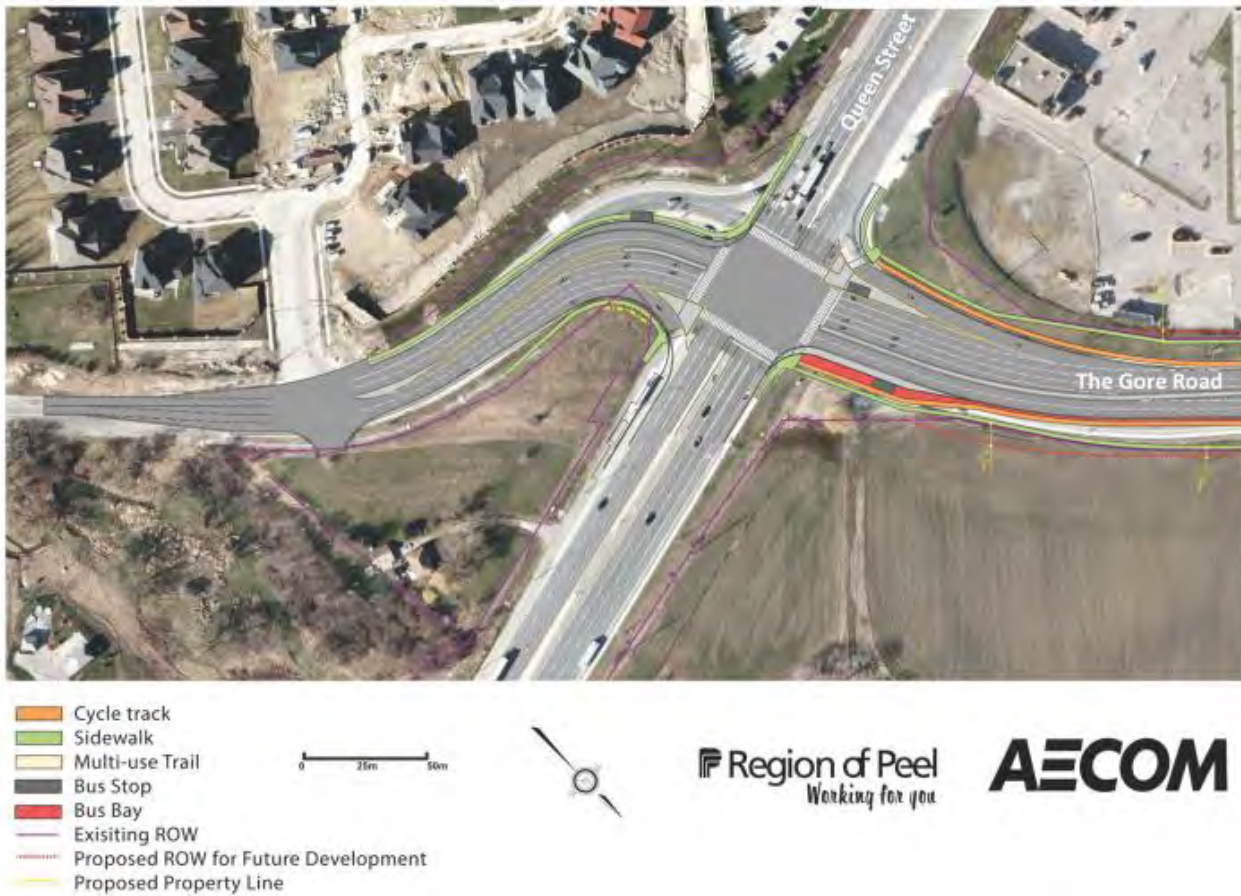
Figure 23 Proposed Queen Street/The Gore Road Intersection Design
