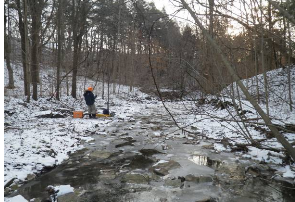
XS 5: View facing downstream. Channel slightly wider than downstream XS's. Scour along right bank resulting in leaning trees and exposure of roots.
