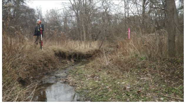
XS 10: View facing downstream. Note bank erosion along outside meander bend (left bank). Right bank has gradual slope.
