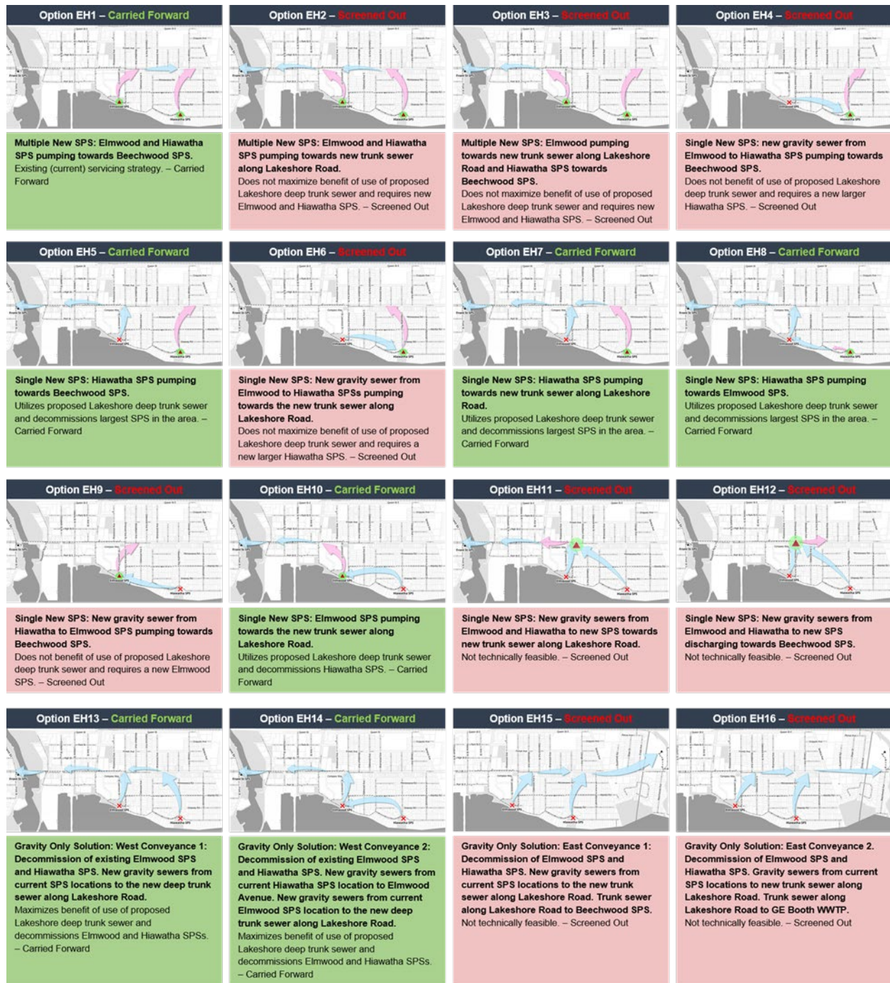
Figure 6-14. Elmwood and Hiawatha SPSs Long List of Conceptual Servicing Alternatives and Screening
