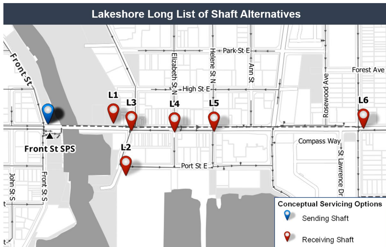
Figure 6-6. Lakeshore Sewer Sending and Receiving Shaft Alternatives
