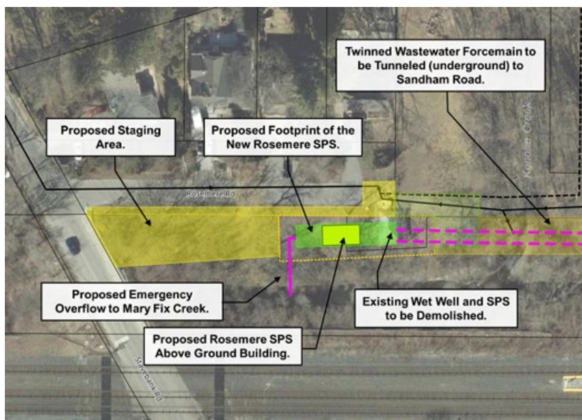
Figure 8-6. Rosemere Road Staging Area (ROS_1)
